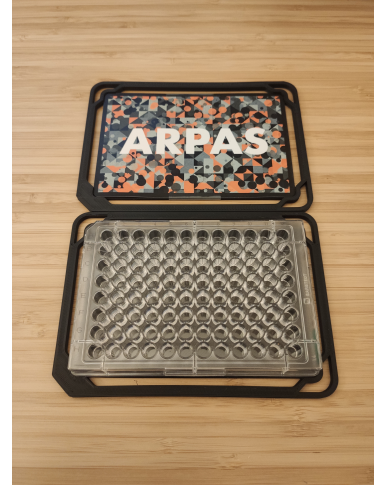
(c) Microplate placed on top of connected frames ready for use in ARPAS v2.
