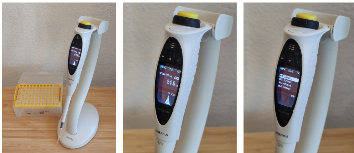
(a) Picus NxT 5-120 \mu L with Optifit Tip Box. (b) Pipette screen showing selected volume (24 \mu L) and pipetting speed (7). (c) Pipette screen showing the four volume presets accessible via the three-striped button.
