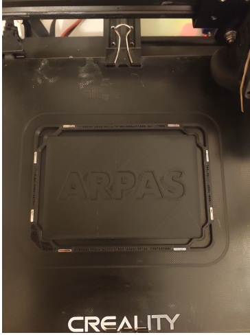
(a) In-print frame with exposed neodym magnet array.
