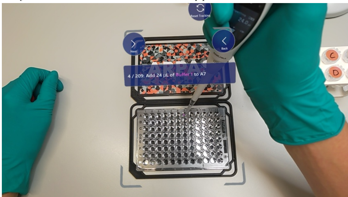
(b) Screenshot of the UI in the fourth-step state, "Dispensing", highlighting the target well for dispensing the set volume of the selected substance with a disc-style indicator at the bottom center of the physical well on the microplate.
