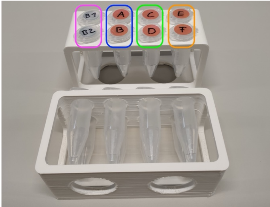
Figure 4.8. Rack for 5 mL micro tubes, labeled B1, B2, A-F. Magenta: pure PBS, Blue: 1/10K, Green: 1/20K, Orange: 1/40K uranine dilution.
