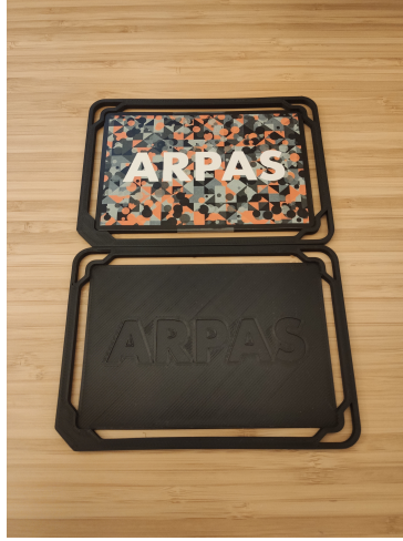
(b) Two frames attached in horizontal orientation, upper frame with Image Target marker.
